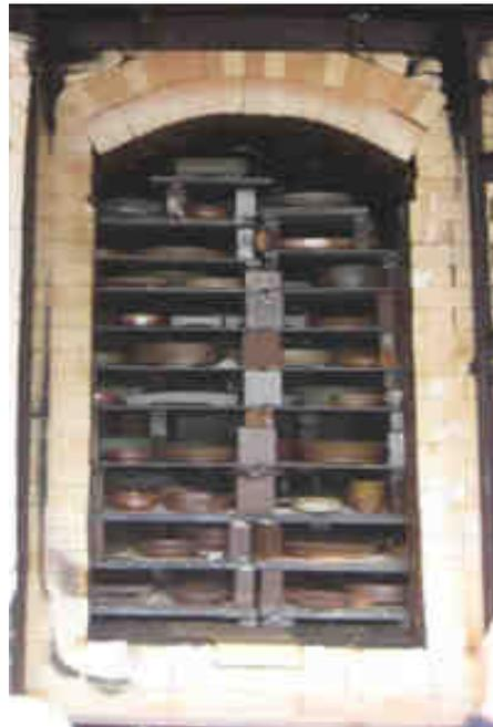
The kiln, built by Ron in 2003 and early 2004 is known as a Phoenix Fast Fire Wood Kiln. The kiln is fired using local Amish milled slabwood of white pine and hemlock and some white oak. It is fired on average for 16 hours, burning a cord and a half of wood to bring the temperature to approximately 2380 degrees Fahrenheit.
